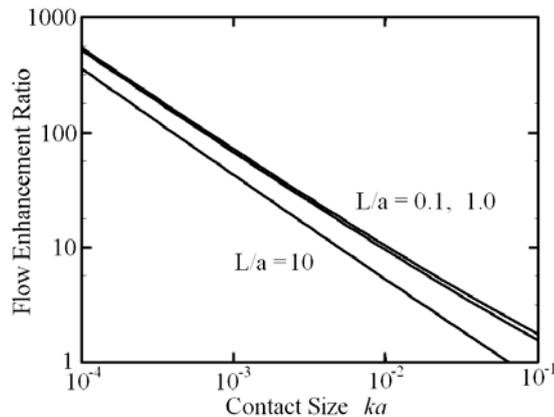
**Figure 4.** Magnitude of the film flow enhancement ratio term of equation (6). This is the ratio of the film flow velocity through the contact to that in the surrounding third sound wave.
