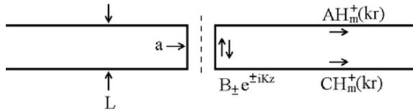
**Figure 1.** Idealized contact point. The ambient wave is on the top plane. Only the scattered components are shown. The contact radius is  $a$  and the length is  $L$ .
